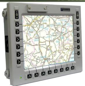
Astronautics' battle-proven Command, Control, and Display Computer Unit (CDU) is specially designed for use in artillery, armored vehicles, and naval vessels. The CDU's open architecture can be tailored to satisfy customer system requirements. The robust 12.1" CDU has a high-resolution display with high contrast and can display graphics or motion video readable in the most demanding direct sunlight conditions and night operations. Features:
