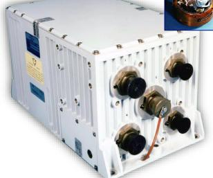
The main sensor of the navigation system is the SEANAV, the INS - Inertial Navigation System senses the ship's angular rates, linear accelerations and provides outputs of heading, pitch, roll and position.
